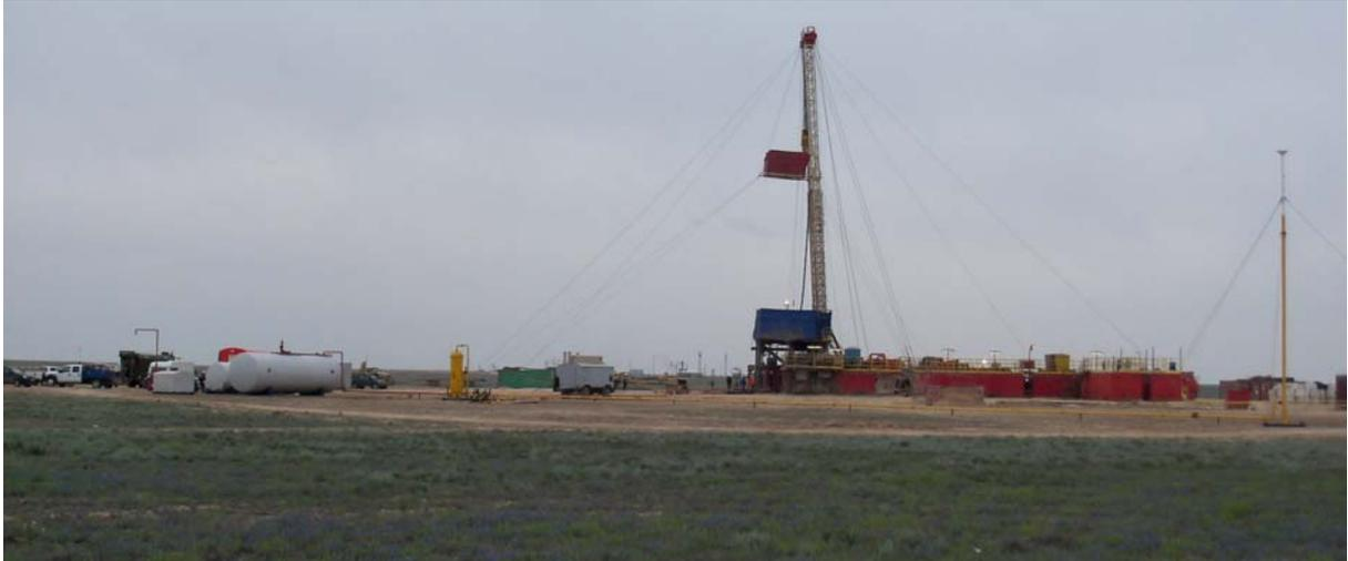
Drilling rig with the well test and temporary production spread in the foreground. Moving from right to left; the gas flare on the far right, the yellow gas-oil-water production separator in the middle left and the white discharge and buffer tanks and off-take arm for discharging oil to customer supplied tanker trucks to the left.
